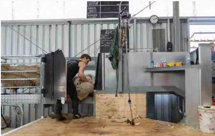
The AWI sheep delivery unit in action. The manual version is featured in this photo; the automatic version is in the photo below.
