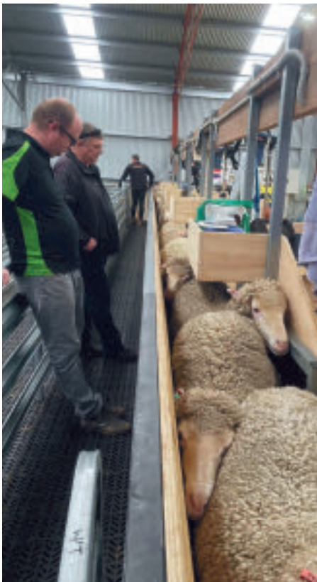
Jarrod King's new shearing setup on display in his shed at the Wool Harvesting Innovation Demonstration Day in October. Behind the shearing stands runs a race, from which shearers can easily remove a sheep (through the gate), thereby greatly reducing the traditional drag.
